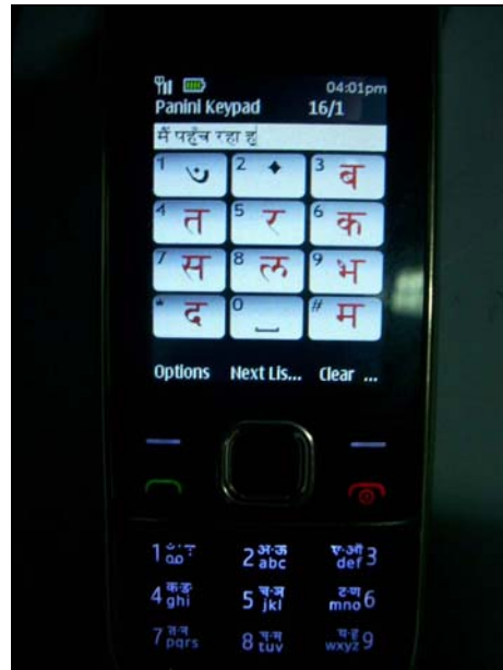
Fig 1. CleverTexting predicting characters that the user could be writing and showing them on the screen from which the user could choose using the keypad or peck directly on the touchscreen The product has been developed for all Indian languages.
